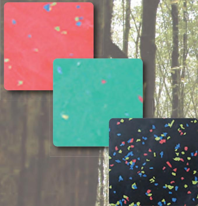
**Natural-FR** is a zero-halogen, low smoke, low toxic rubber compound based on natural rubber.
